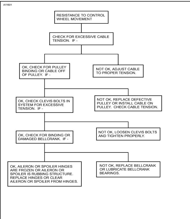
Figure 101 : Sheet 2 : Aileron and Control System Troubleshooting Chart
